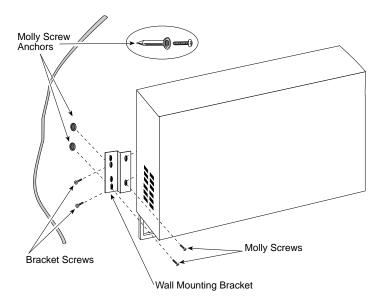
Figure 3-6. Installing the Wall Mounting Brackets
